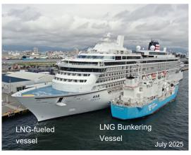
LNG bunkering vessels enable the supply of LNG fuel to ships at Hakata Port.
