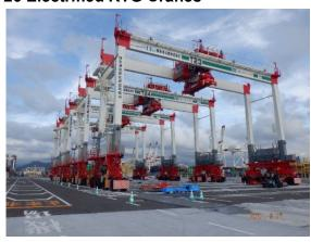
These cranes handle containers in the terminal yard. Electrification has achieved significant energy savings compared to conventional diesel-powered models.
