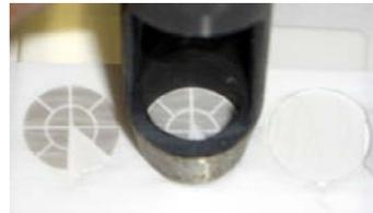
Fig.2 SPM spots are cut 1/8 for daily average measurement (left) and cut out for hourly measurement (center).
