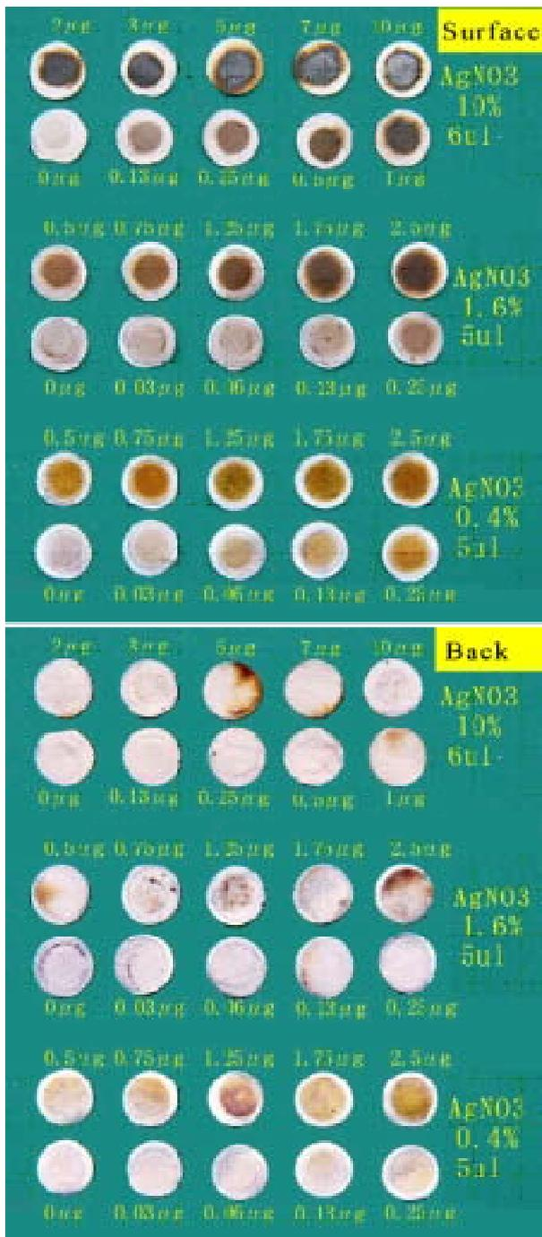
Fig. 2 Coloring situation of having changed the concentration of  $\text{AgNO}_3$  and amount of arsenic
