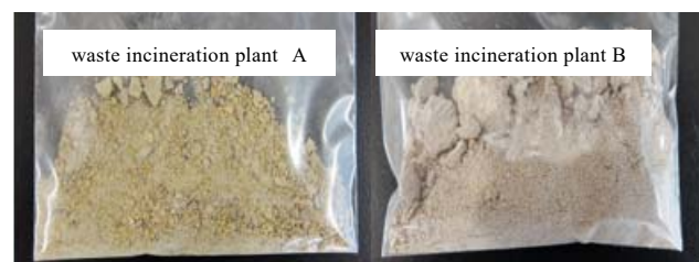
Fig. 1 Fly ash adhering to the boiler water pipe
