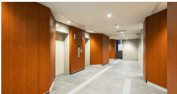
The floor and walls contrast with each other, making it easy to recognize the space. Elevator doors contrast with surrounding walls and are easy to recognize.
