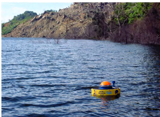
◆ Indonesia/Ambon Island Land slide dam water observation (Buoy-type water level gauge )
