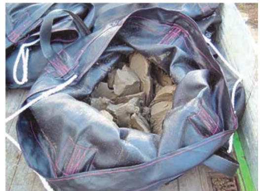
↑ Conditions of sludge inside Eco Pouch before moving out About 24 hours later, the sludge changed into dewatered sludge cake
