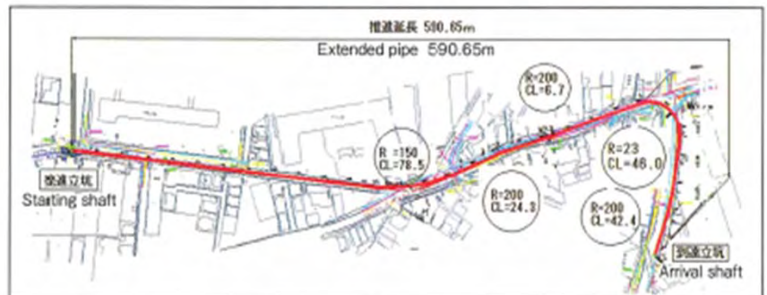
曲線施工 Curved pipeline construction
