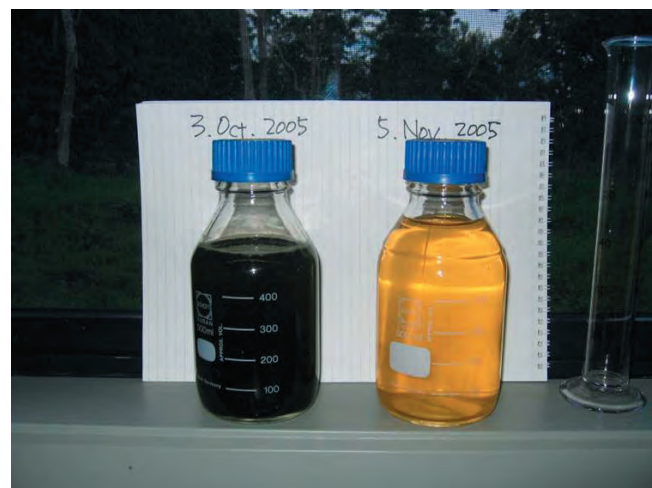
Leachate before improvement and improved Leachate (2005)
