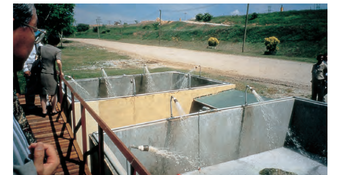
Adsorption processing using activated waste carbon
