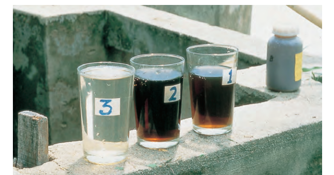
Leachate (1: Untreated, 2: After aeration, 3: After filtration and adsorption processing)
