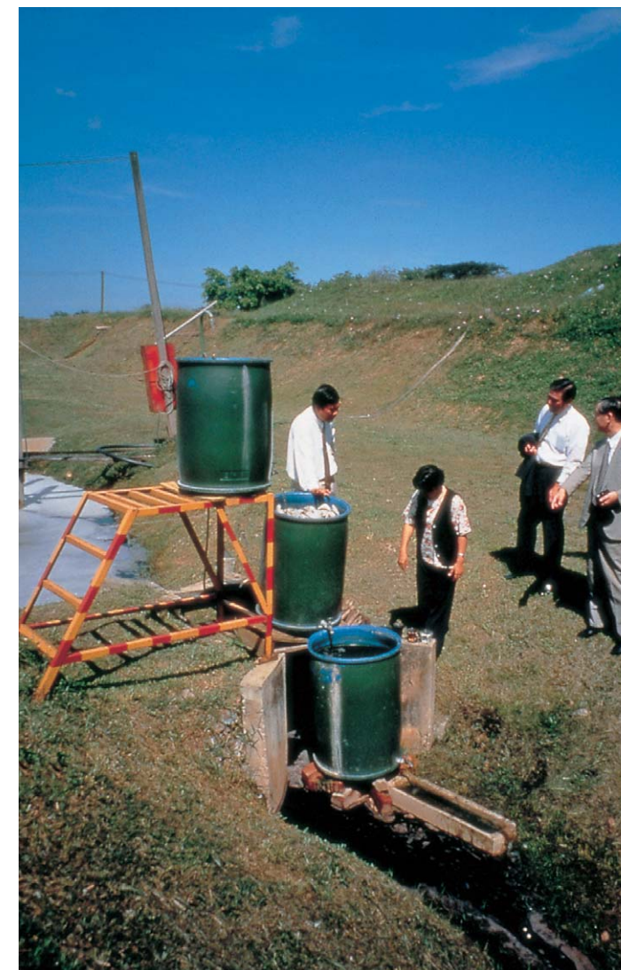
Leachate treatment facility (pilot plant)
