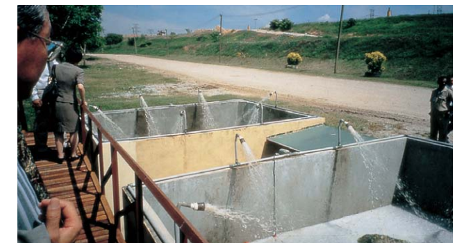
Adsorption processing using activated waste carbon
